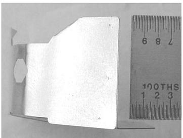
The angle between the face and base (back) of the ribbon shield must be perpendicular. Ribbon shields are made of thin stainless steel and if bent can cause poor print quality or snag the ribbon fabric.
