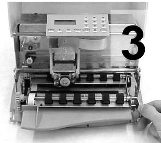
Rotate lift ring forward to lift
