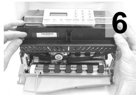
Rotate cartridge into place and snap in.
