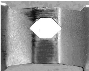
Ribbon shield at end of life. Face is scored. There is no visible damage to the six-sided opening but a breach is imminent. This shield may begin to snag documents.
