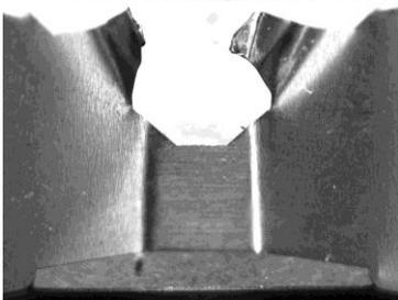
Damaged ribbon shield. One side of the six-sided opening is missing. This ribbon shield will streak and tear every document and may scratch the platen.
