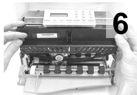
Rotate cartridge into place and snap in.
