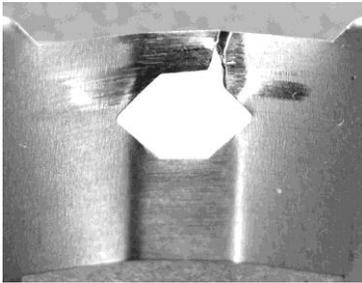
Damaged ribbon shield. There is a breach in the six-sided opening. This ribbon shield will streak and tear documents.
