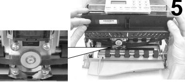
Slip ribbon over and behind guide plate tabs. Rotate cartridge into place and snap in. Rotate cartridge drive gear clockwise to align and take up ribbon slack. **Push ribbon shield and ribbon guide plate up.** Lower carriage into operating position. Close cabinet.
