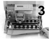
Rotate lift ring forward to lock carriage in the up position.
