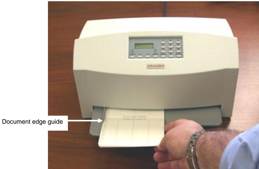
Insert a passbook or other document by placing the left edge of the document against the edge guide and gently move it into the printer. Release the document when the feed rollers begin to feed it into the printer. The printer will straighten the document (automatic alignment) before printing if necessary.
